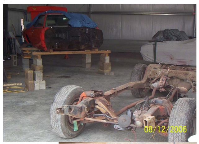
The chassis was completely taken apart, down to the last nut and bolt and bracket, and cleaned with chemicalstripper or a wire brushcup drill attachment, or both. The body had the interior was re-done, and the body was mated back onto the re-done chassis in mid-December.
